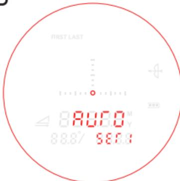
This mode can measure the distances to both the nearest and the farthest targets simultaneously.
