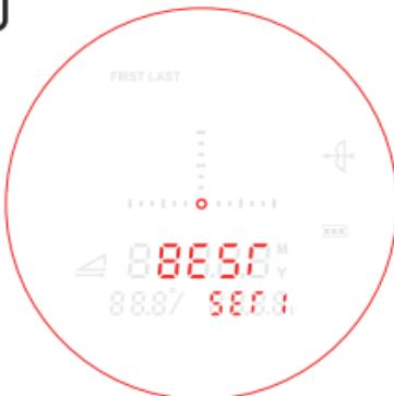
This mode is recommended when there are no obvious obstructions in front of the target and no significant interference from the background. It offers a measure range up to 2,000 yards for most targets, which under normal ranging conditions have medium reflectivity.
