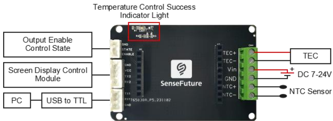
Figure3 TEC103/TEC103L Adapter Board Wiring Diagram
