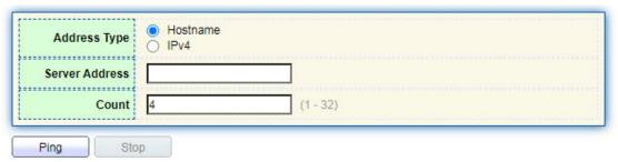
2. Click the "Ping" to accept the packet-transmitting test from system to verify address validity, and output the result as follows:
