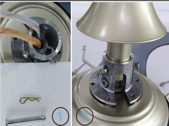
**Step 5:** as shown in the picture, take out the safety pins, put the light pole into the light body to wear the safety pins and tighten the screws to fix.
