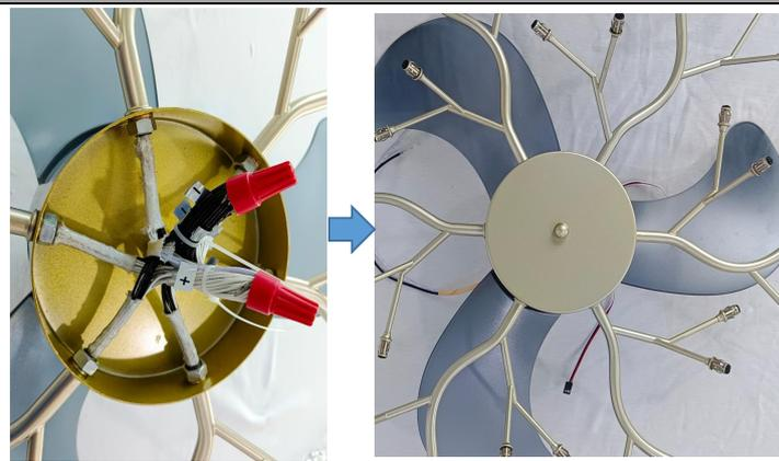
**Step 3:** as shown in the picture wiring, tied with a cable tie and screwed on the wire cap, and screw the round piece back (black to black, white to white).
