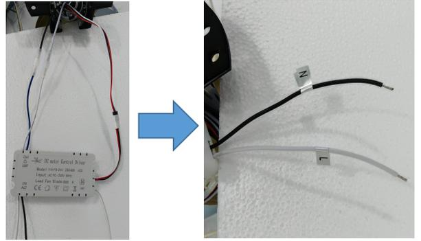
Step 7:as shown in the picture wiring (black and white wire access to the power cord) .
