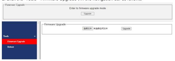
Note: After clicking OK, do not power off during the upgrade process, stay on the upgrade page for about 1 minute until the upgrade is complete
