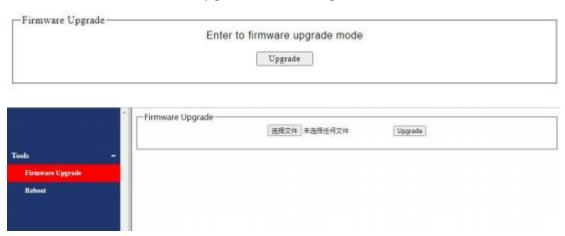
Note: After clicking OK, do not power off during the upgrade process, stay on the upgrade page for about 1 minute until the upgrade is complete
